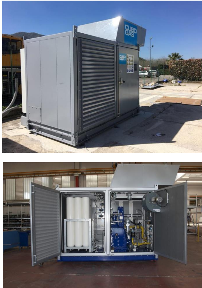
Figure 142: CNG compression and storage module Source: Cubogas
