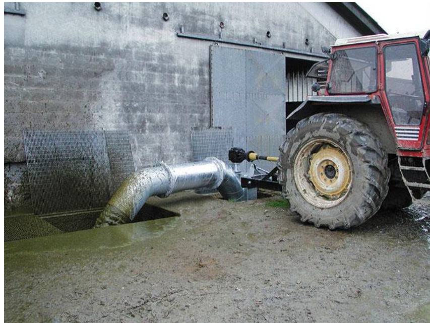
Figure 166: Liquid phase pumping Source: Veneroni-srl.it
